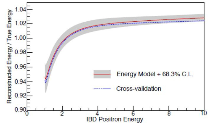
**Nominal energy model:** fit to mono-energetic gamma lines and  $^{12}\text{B}$  beta-decay spectrum
