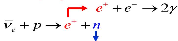
Delayed signal, Capture on Gd (8 MeV),  $\sim 30\mu\text{s}$
