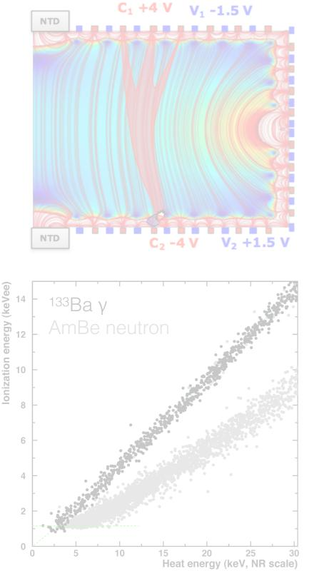
FID Ge crystals: event ID from measurements of ionization and phonon energies
