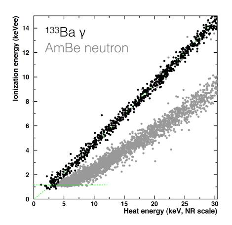
FID Ge crystals: event ID from measurements of ionization and phonon energies
