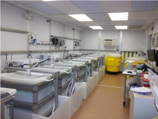
Electroforming Baths in TCR
