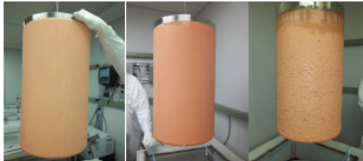
Inspection of EF copper on mandrels
