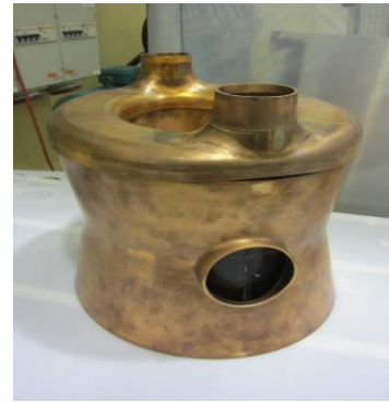
CERN Cavity production for beam tests (Established manufacturing procedures)
