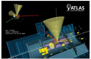
Display of a  $t\bar{t}$  candidate event from proton-proton collisions recorded by ATLAS with LHC stable beams at a collision energy of 13 TeV. The red line shows the path of a muon with transverse momentum around 140 GeV through the detector. The green line shows the path of an electron with transverse momentum around 170 GeV through the detector. The green and yellow bars indicate energy deposits in the liquid argon and
