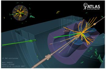
Display of a p-p collision event recorded by ATLAS on 21 May 2015 at a collision energy of  $\sqrt{s}$  =13 TeV. Tracks reconstructed from hits in the inner tracking detector are shown as arcs curving in the solenoidal magnetic field and green bars are proportional to the energy deposited in the electromagnetic calorimeter. A high energy electron and positron are identified with an invariant mass consistent with that of a Z boson.
