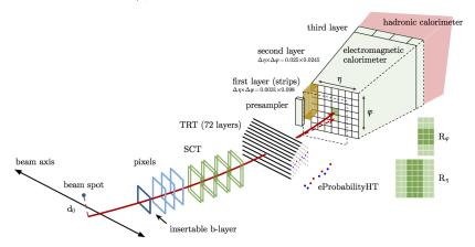
A combination of information from the Inner Detector (track) and the Electromagnetic Calorimeter (energy deposit, cluster).
