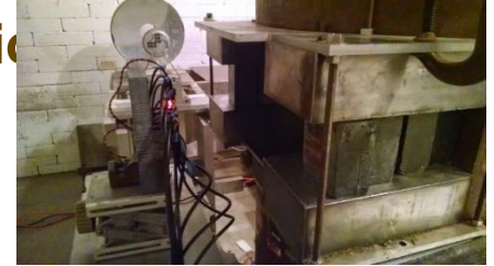
Repeater board @ Co-60 source location
