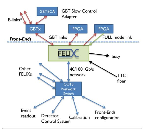
\* E-link: variable-width logical link on top of the GBT protocol. Can be used to logically separate different streams on a single physical link.
