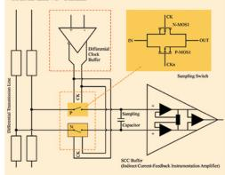
The above figure shows the RFpix sampling cell (SC) schematic. The SC structure follows a differential configuration with the two SC switches denoted as P and N respectively. Both switches are driven by a local differential clock driver, which ensures fast rise times (31ps) and prevents clock skew.
