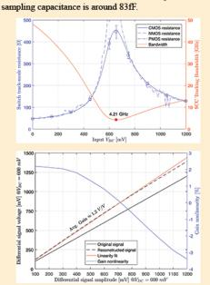
By observing the differential output, the sampling error becomes almost symmetric. By considering the original signal amplitude versus the reconstructed sampled signal amplitude, the amplitude dependent offset voltage turns into a virtual gain of the SC.
