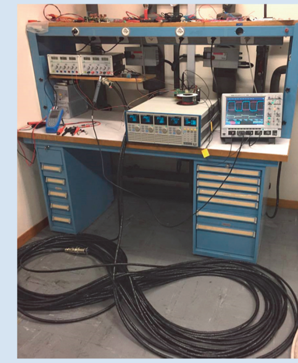
Test setup with proto cables and electronic loads
