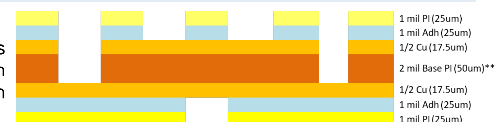
Figure 12 Tape stackup using polyimide layer with double metal.
