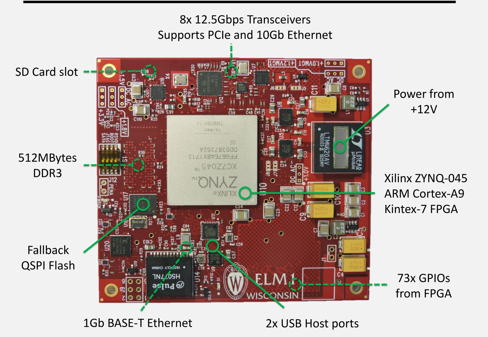
Short for ELM, the Embedded Linux Mezzanine is intended to be used as the blade's on-board computer and its primary access point. It features a dual core ARM processor packed inside a high-end Xilinx ZYNQ System-on-Chip (SoC) running a full-fledged Linux distribution.
