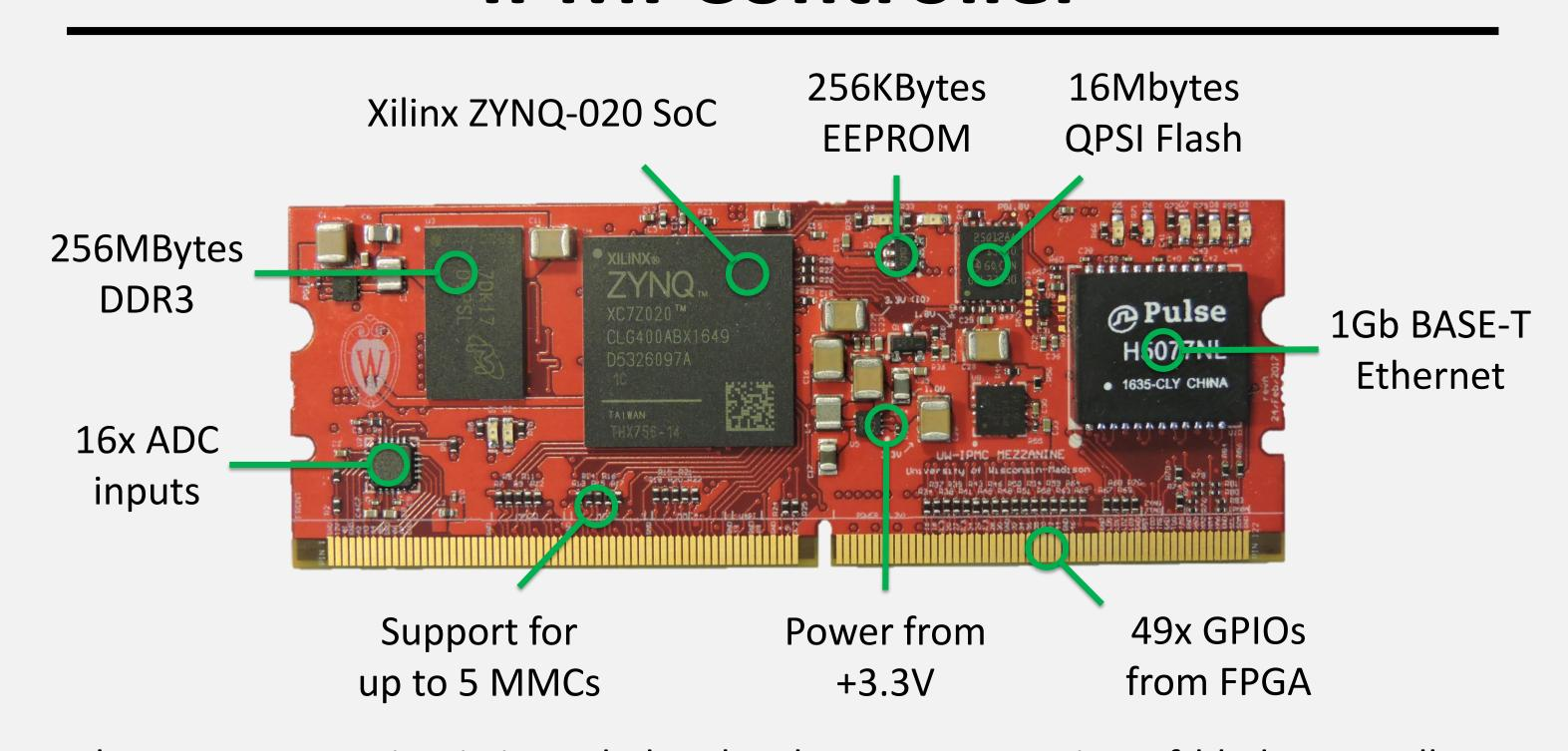
The IPMC mezzanine is intended to be the next generation of blade controllers that communicate with ATCA Shelf Managers (ShMC). It is part of the PICMG 3.x specification and each blade needs to have one of such controllers. They are responsible for doing blade related health checks (e.g. temperature, voltages) and to act in case of problems, such as over-temperature or over-voltage.
