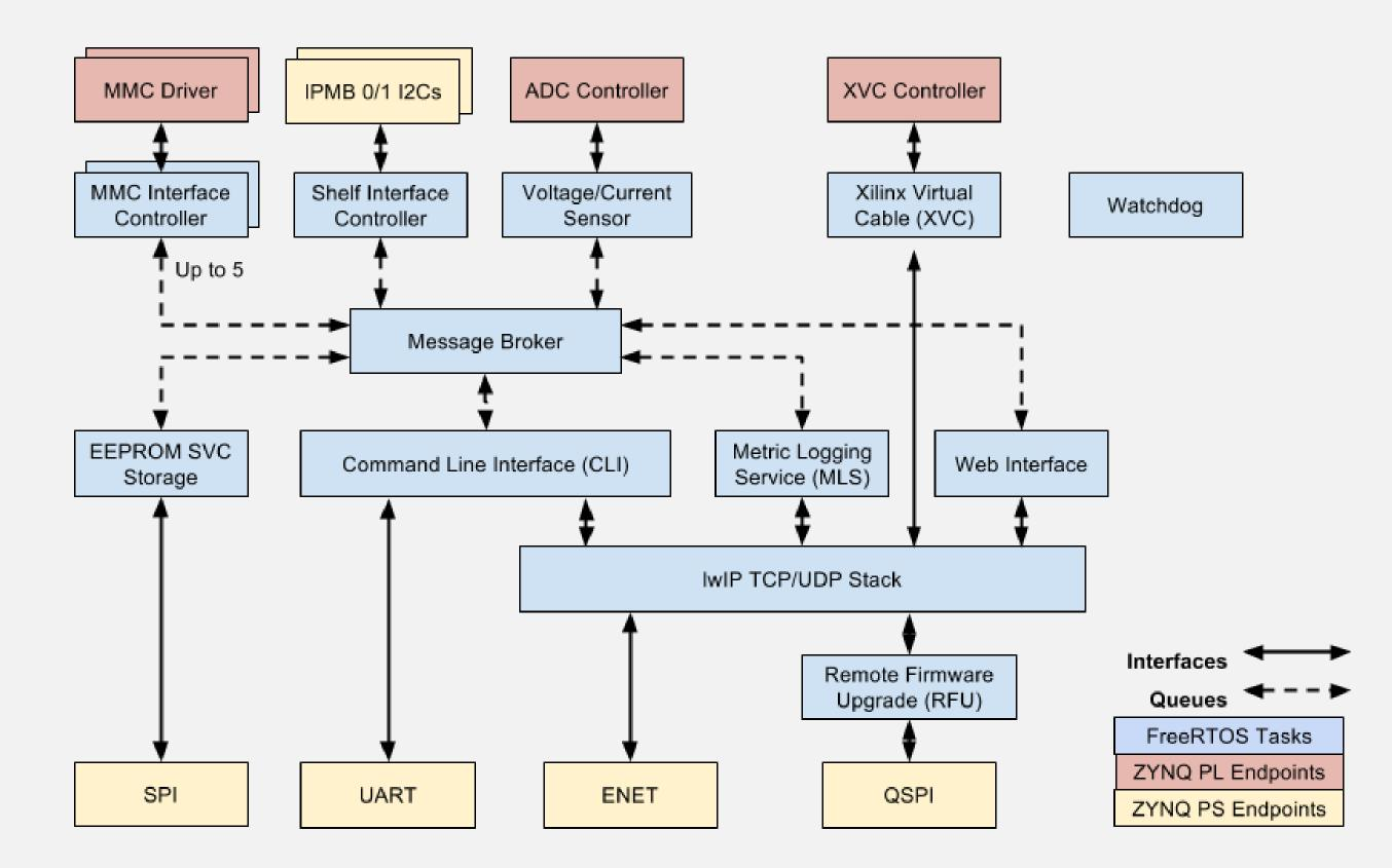
Five independent Modular Management Controller (MMC) interfaces allows the IPMC to manage Advanced Mezzanine Cards (AMCs), this preventing bus locking in case one AMC fails. For expandability, 49 GPIOs are available at the mezzanine connector and wired to the FPGA section, allowing the IPMC to interface with power, monitoring or management related components on the ATCA blade. They can also be used to add more MMC interfaces.
