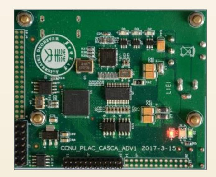
The Adapter card named CASCA\_AD card, edged-mounted with the CASCA card, is in charge of digitizing the output from the CASCA card and driving the ASIC. A low-power FPGA chip, a 12-bit ADC and a multi-output clock generating chip are mounted on the CASCA\_AD card.
