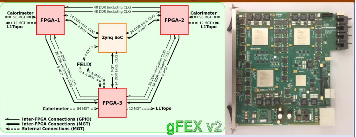
FEX v2 is a full function prototype with three Virtex UltraScale FPGA and one ZYNQ FPGA.
