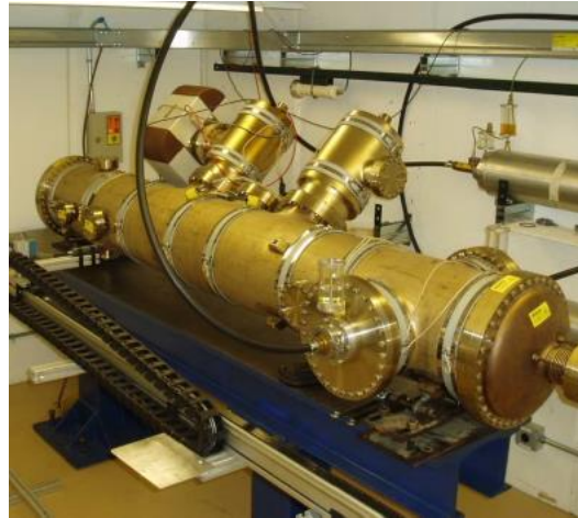
Tevatron electrostatic separator in the vacuum chamber
