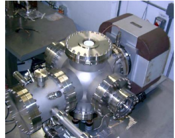
DC high voltage field emission test stand
