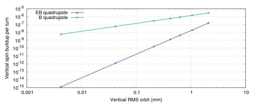
• The MDM spin transparent quadrupole considerably reduces the effect of misaligned vertical orbit onto the vertical buildup.
