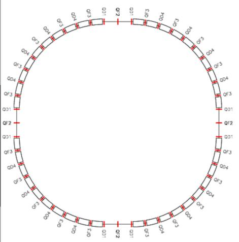
Lattice developed in [1] for proton EDM and using here combined EB deflector.
