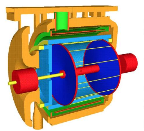
Be beam pipe (0.5 mm thick) Instrumented permanent magnet quadrupoles (32 PMT's)
