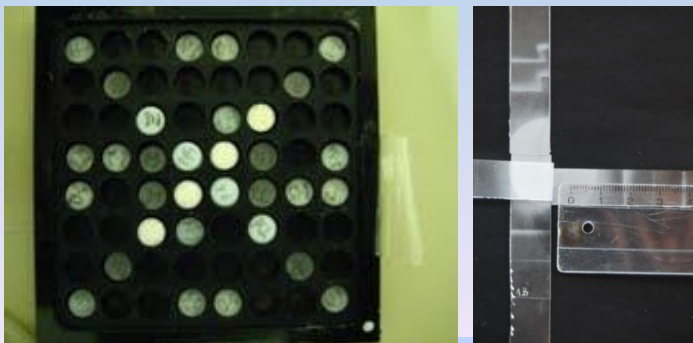
TLD and PADC in proton beam
