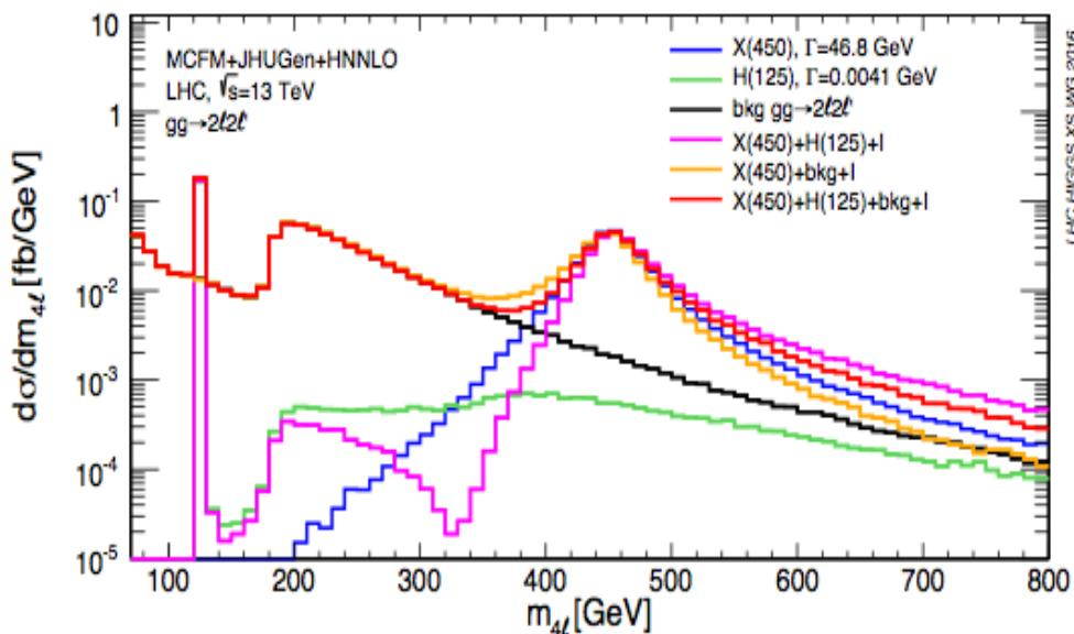
→ Model can also be extended for an additional Higgs of arbitrary  $\Gamma_X$  with interference to SM Higgs or bkg (example from gluon fusion)
