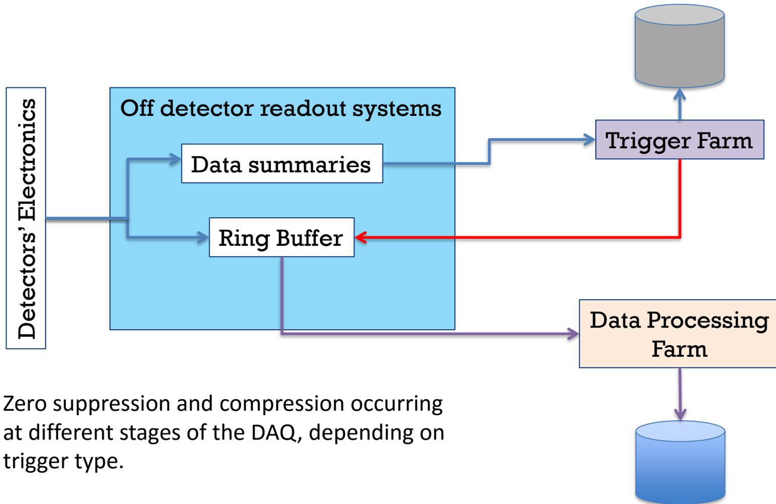
Zero suppression and compression occurring at different stages of the DAQ, depending on trigger type.
