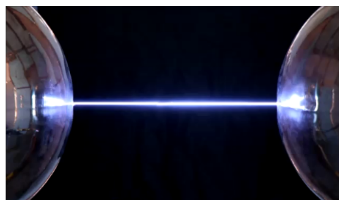
Laser filament-assisted guided discharge between two spherical electrodes.
