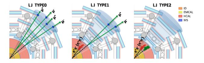
Muons without associated inner detector tracks are more susceptible to cosmic backgrounds, beam halo. Specialized trigger needed in both cases
