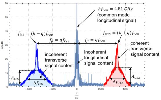
• Extract the chromaticity from the measured Schottky side  $b_{\Delta f_{lsb}}^{\Delta f_{usb}} + a_{f_{usb}} + q \approx \eta h \frac{\Delta f_{lsb} - \Delta f_{usb}}{\Delta f_{lsb} + \Delta f_{usb}}$
