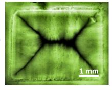
MOI images of sample 1 [1]. The film was zero-field cooled to 20 K and a magnetic field was subsequently applied perpendicular to the film.
