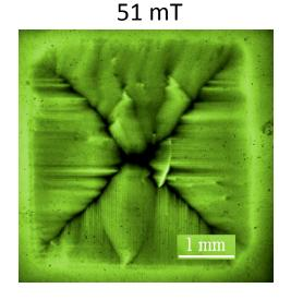
Optical (left) and MOI images (centre, right) of sample 2 [1]. The film was zero-field cooled to 20 K and a magnetic field was subsequently applied perpendicular to the film.
