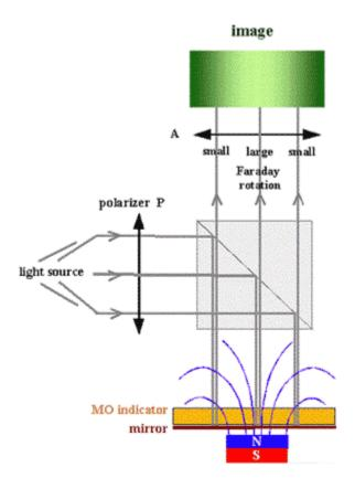
Magneto-optical imaging (MOI) is used for visualising magnetic flux in superconductors.
