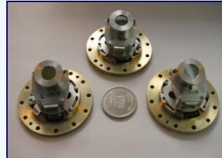
Particle detectors (HPGe, Si PIN diode, PIPS) operating at  $\sim 10\text{K}$  and  $1\text{T}$
