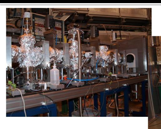
Vacuum testing, initial bake-out of UHV section reached <5e-9mbar (limit of the gauge) in the interaction region.
