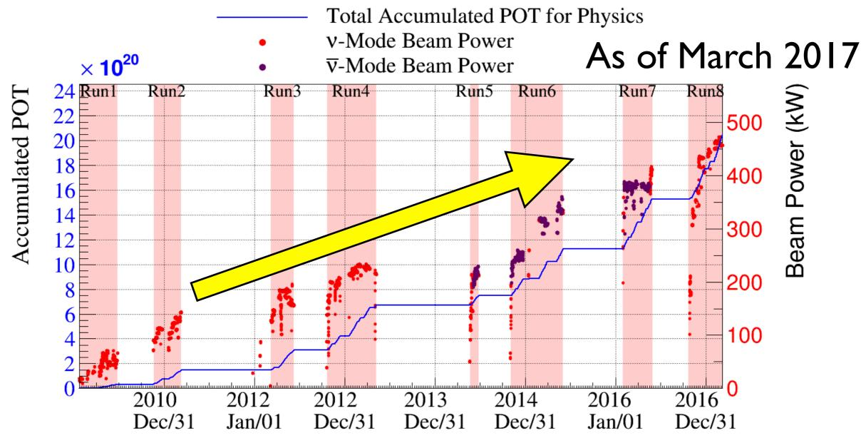
Operated with 470kW, still increasing towards >500kW Total POT exceeded 2×10<sup>21</sup> (doubled in ~2 years)
