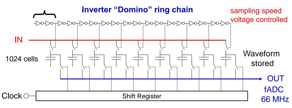
it works like a time stretcher, but with no deterioration of signal / loss of information: sampling ~ 5 GHz range digitization ~ 50 MHz range
