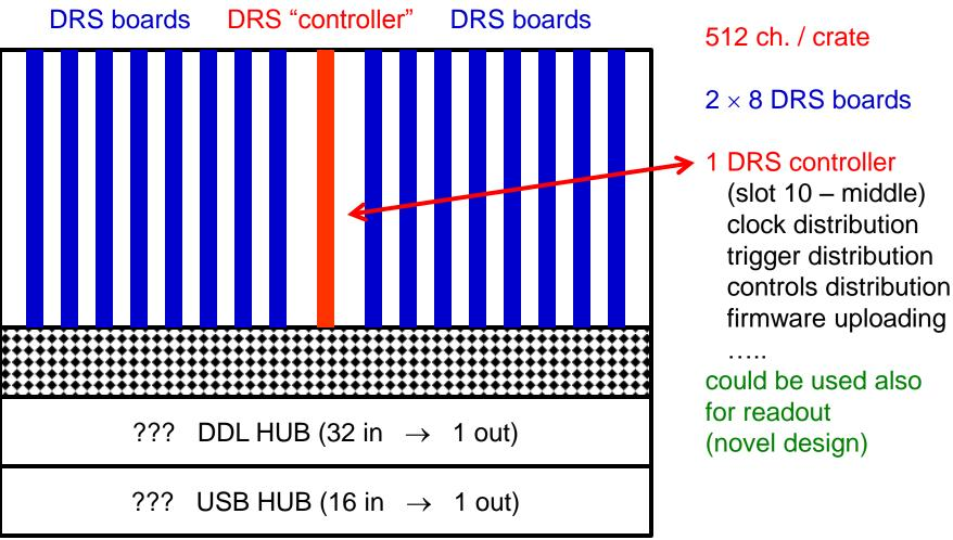
with on board clock generation (controller) can have a stand alone system with 512 synchronized channels and USB 3.0 readout
