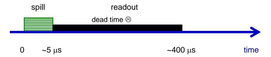
Buffer depth and sampling time driven by "active" window and signal speed (for good timing, 4 or 5 samples on the rising edge)
