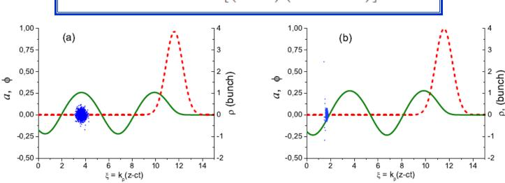
At the entrance of the matched plasma channel, the laser pulse envelope was Gaussian in both longitudinal and transverse directions with laser wavelength  $\lambda_0 = 0.8 \, \mu m$ , amplitude  $a_0 = 0.964$  and FWHM pulse duration  $\tau_{FWHM} = 50 \, \text{fs}$ , and waist radius  $r_0 = 68.2 \, \mu m$
