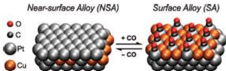
Figure 1. Illustration of (left) the CuPt NSA and (right) CO-induced Cu surface segregation and the novel SA resulting from it.
