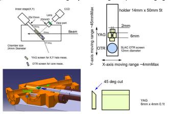
Horizontal slices are cut by 45 deg to avoid edge effects (horizontal insert)
