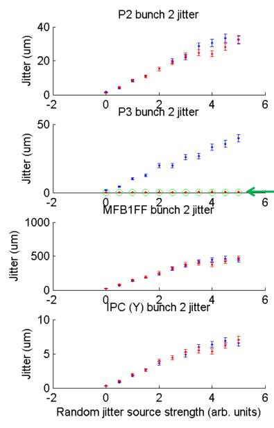
feedback off jitter (blue) feedback on jitter (red)
