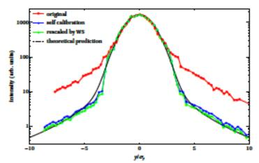
Beam profile after rescaling is comparable with estimation, while both of them agree well with halo predicted by BGS theory/simulation!
