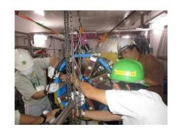
Installation is now completed. Both magnets are mounted on micrometric tables. First electrical checks at installation were done with a temporary power supply all tests were positive.
