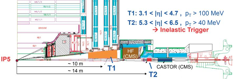
**Roman Pots:** elastic & diffractive protons close to outgoing beams **> Proton Trigger**
