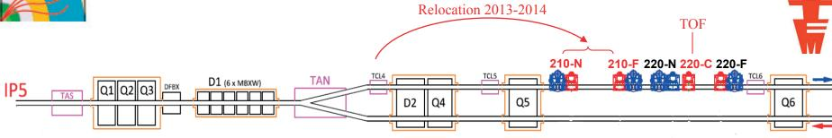
**Upgrades for operation at high luminosities** within the CMS-TOTEM Precision Proton Spectrometer (CT-PPS) project for running in all standard LHC fills at low β\*
