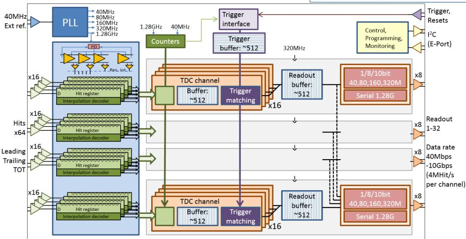
64 channels, 3ps or 12ps time binning, 100us dynamic range 64 channels, 3ps: ~1W; 64 channels, 12ps: ~0.5W; 32 channels, 12ps: ~0.3W
