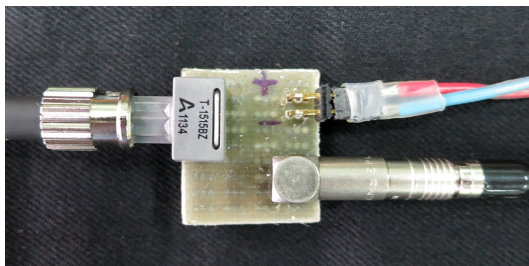
Figure 6: Photo (left) and simplified schematics (right) of the LED pulser
