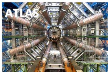
**ATLAS** is a general-purpose detector. Six subsystems, in layers around the collision point, record the paths, momentum & energy of particles to identify them.
