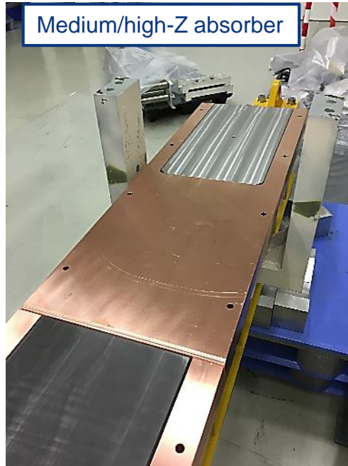
Graphite inside the CuCrZr core
