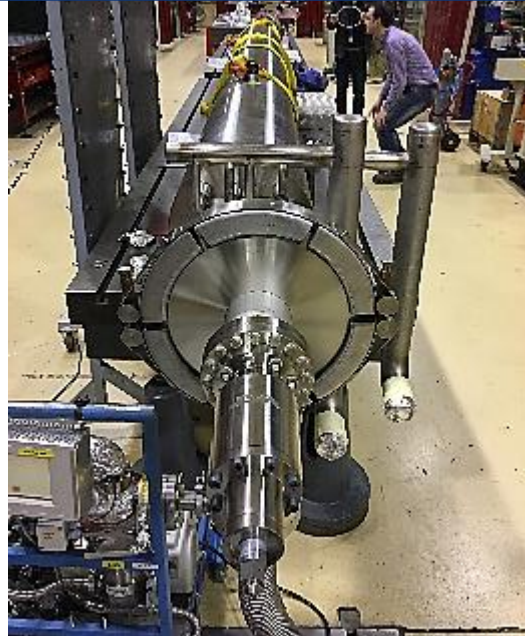
Final leak detection (downstream)
