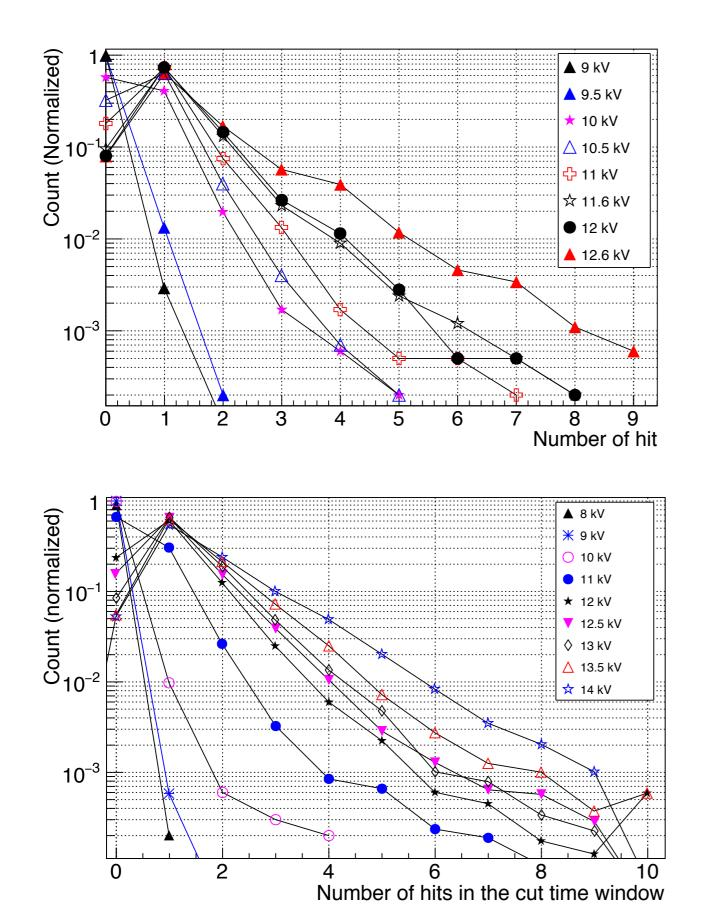
For 4 gas gaps MRPC at 12 kV, around 75% of the events recording a single hit. About 19% of the events exhibited more than one hit
