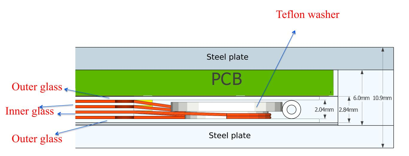
4 gas gaps MRPC: 3 inner glass sheets (280 μm), 2 outer glass sheets (400 μm) 5 gas gaps MRPC: 4 inner glass sheets (280 μm), 1 outer glass sheet (280 μm), 1 outer glass sheet (400 μm)
