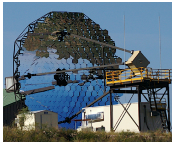
Cherenkov telescopes Like VERITAS and CTA
