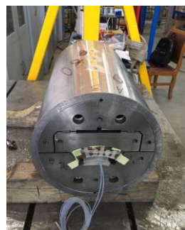
Sextupole coil and bladder+key test assembly
