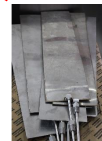
Sextupole coil and bladder+key test assembly
