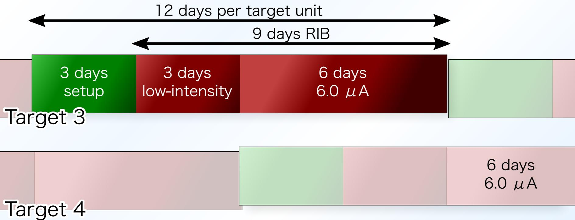
Protons used per target 36  $\mu$ A.days (5e19)
