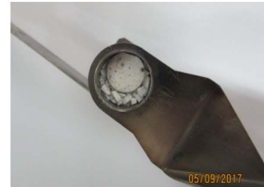
MgO discs in the target tube
