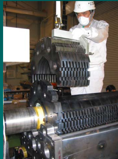
Top Yoke Installation
