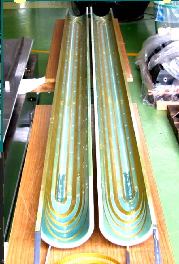
Mirror-symmetry Top & Bottom coils of the prototype
