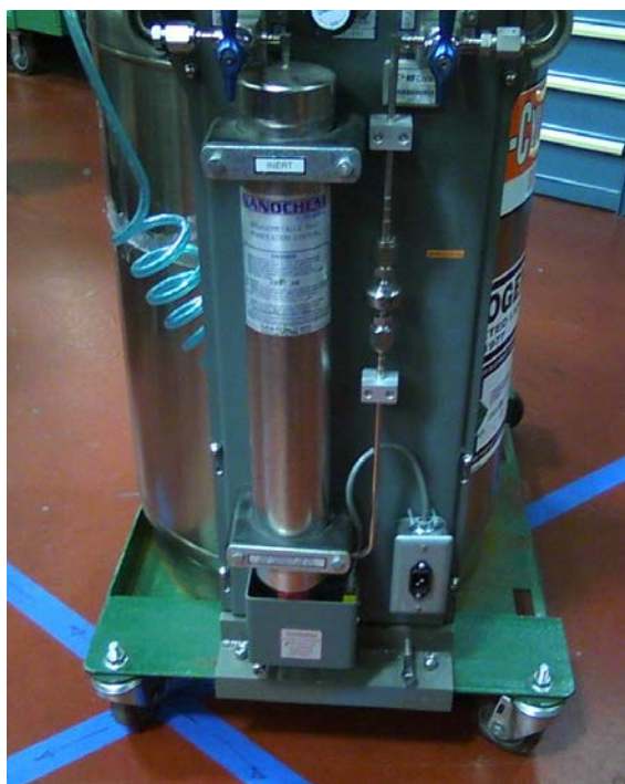
Purifier mounted to an LN dewar at the LBL Advanced Light Source
