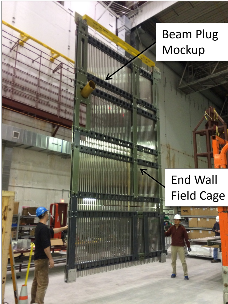
End Wall Field Cage with Beam Plug Mockup at Ash River Trial Assembly
