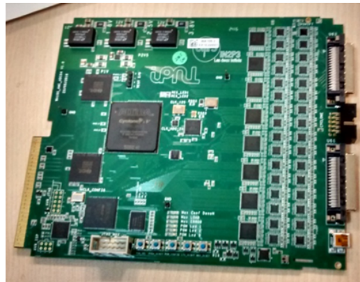
FIG. 55: 64 channels microTCA digitization cards. A preproduction sample of 20 cards is currently operational on LAr-Proto.
