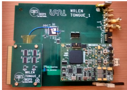
FIG. 59: microTCA White-Rabbit slave card for timing and triggers distribution
