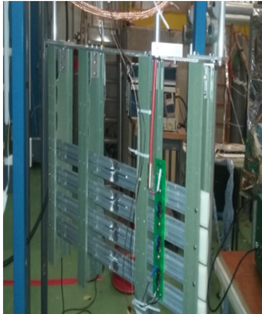
FIG. 46: Mechanical mock-up used at CERN to test the shape of the clipping profiles and the functionality of the field cage electrical elements, as well as the trial fit and cleaning of all sub-module elements
