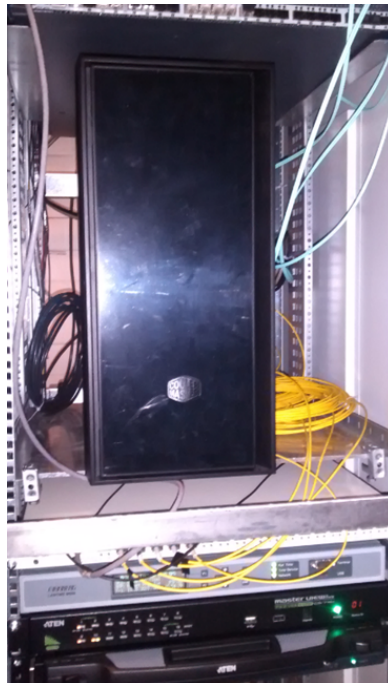
FIG. 60: Full timing/trigger system already deployed on LAr-Proto including the GPS receiver, the White-Rabbit grand master and the trigger PC hosting the White-Rabbit time-tagging card
