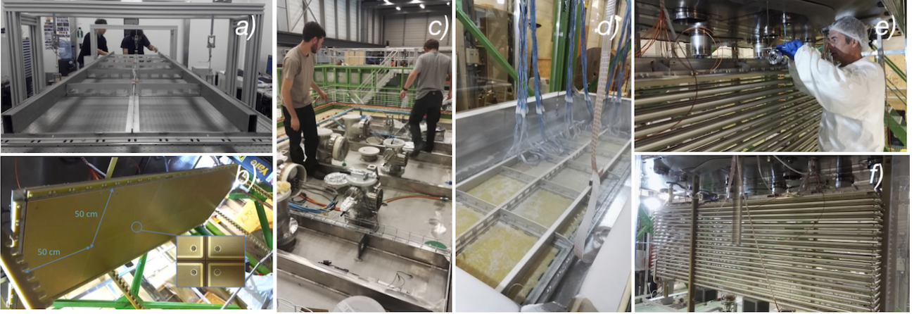
FIG. 7: Main step of the detector assembly. The CRP is first assembled in the clean room (a) then suspended under the top-cap with the motorised suspension feedthroughs (b,c). The CRP underwent a shock cryogenic test in liquid nitrogen bath (d) and lifted back into nominal position so that the drift cage and other detector components could be installed (e,f).
