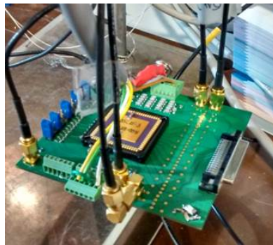
FIG. 51: Final version of the double-slope cryogenic ASIC amplifier submitted for production in October 2015 and tested at the beginning of 2016.
