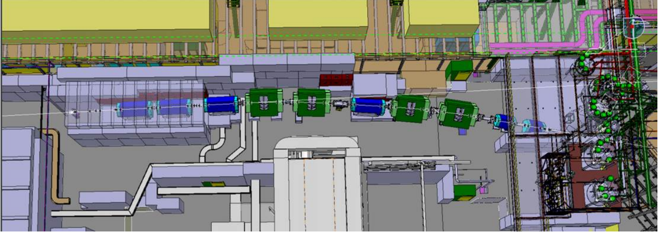
FIG. 22: 3D CAD view of the H2-VLE beam-line
