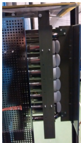
FIG. 41: Prototype built at CERN in order to test the field cage design based on the extruded open aluminum profiles
