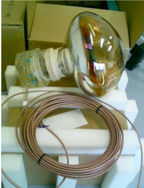
RG-303 attached to one of the Double-Chooz PMT
