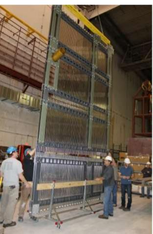
Top three sections are bolted to the last section
