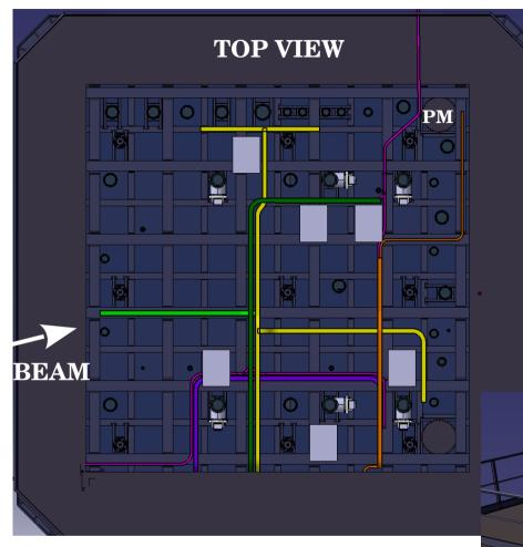
Yellow tray: temperature profile and cryostat temperature sensors
