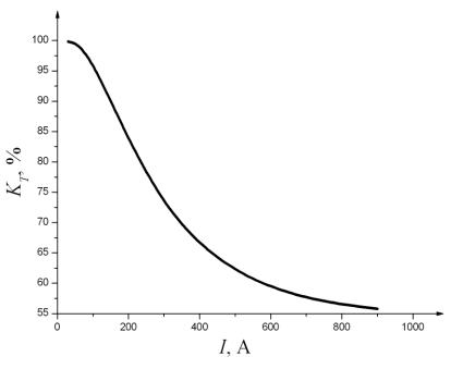
The capturing coefficient vs. bunch peak current for the case of using the photocathode (*half of lost particles forms back-current!!!*)
