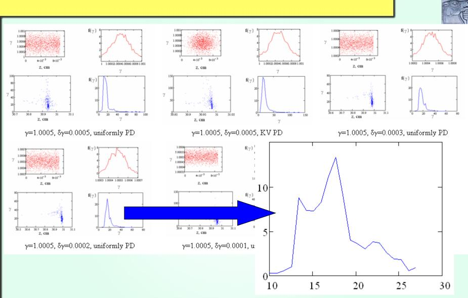
Phase portraits and energy spectrums (initial by red, output by blue) for different initial conditions,  $E_z$ =800 kV/cm, the bunch charge 6 nC, uniformly and KV initial phase distributions, B=0.2 T.
