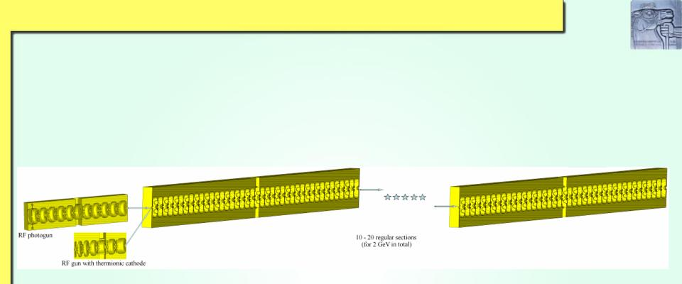
Possible scheme of linac layout: RF gun with thermionic cathode is option for high intensity drive bunches production for  $e^{-/e^+}$  conversion and photogun for <1 nC high quality bunches generation (close to SuperKEKB new injection scheme).
