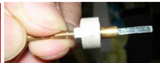
Synthesized rock salt 2 \times 2 \times 10 \text{ mm}^3
