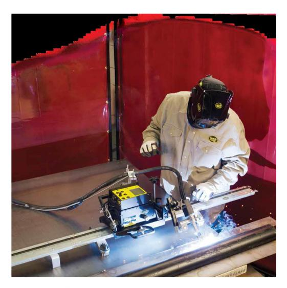
Bug-O Systems – Automated Cutting & Welding System: Modular Drive System
